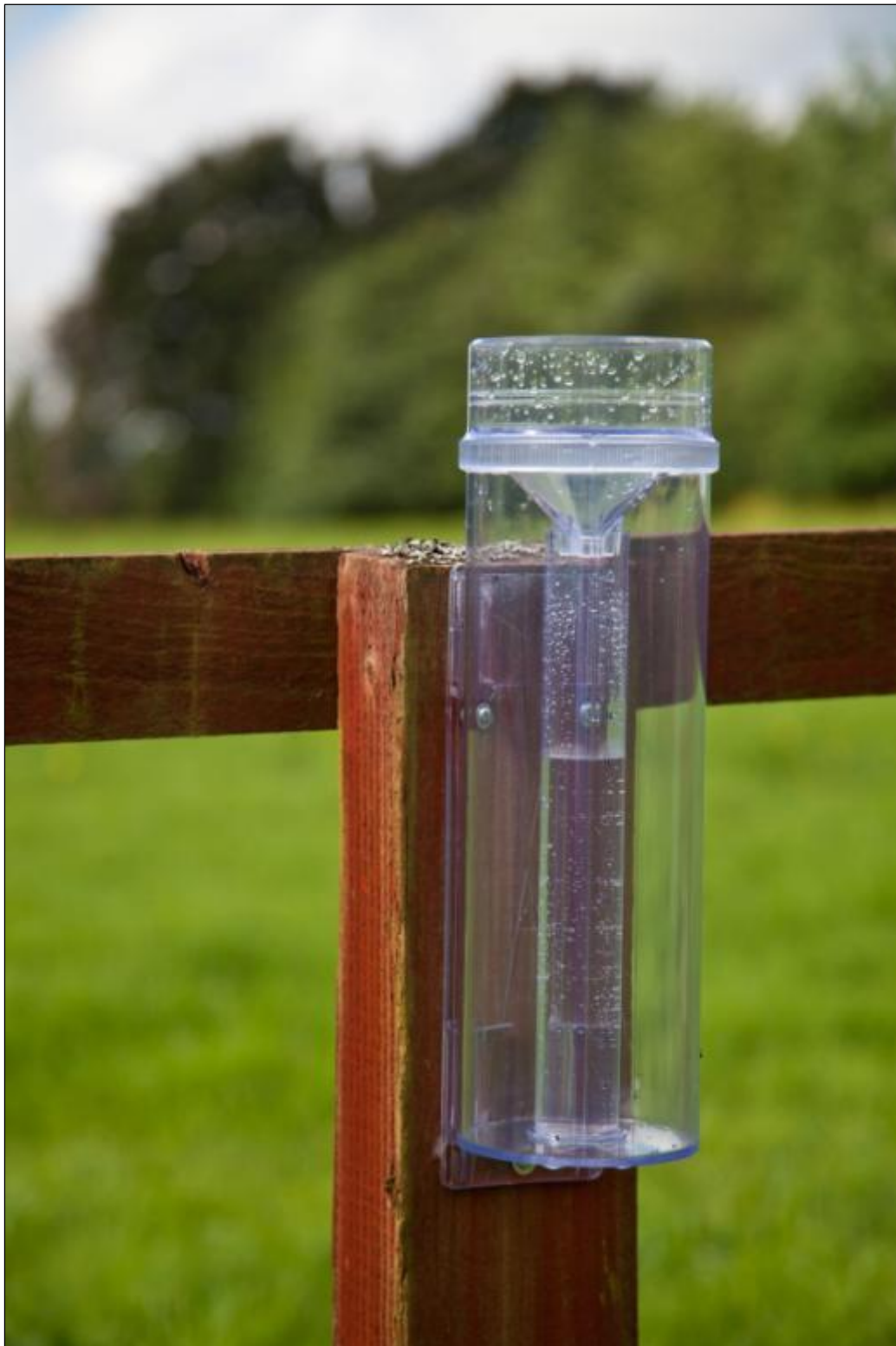
Figure 1 - The CoCoRaHS gauge used in this comparative trial. It is mounted on a fence post with its rim at 125 cm above ground level. Note the splashes from falling raindrops within the upper part of the measuring cylinder, and undrained droplets remaining within the funnel. Photograph taken on 14 August 2012.
