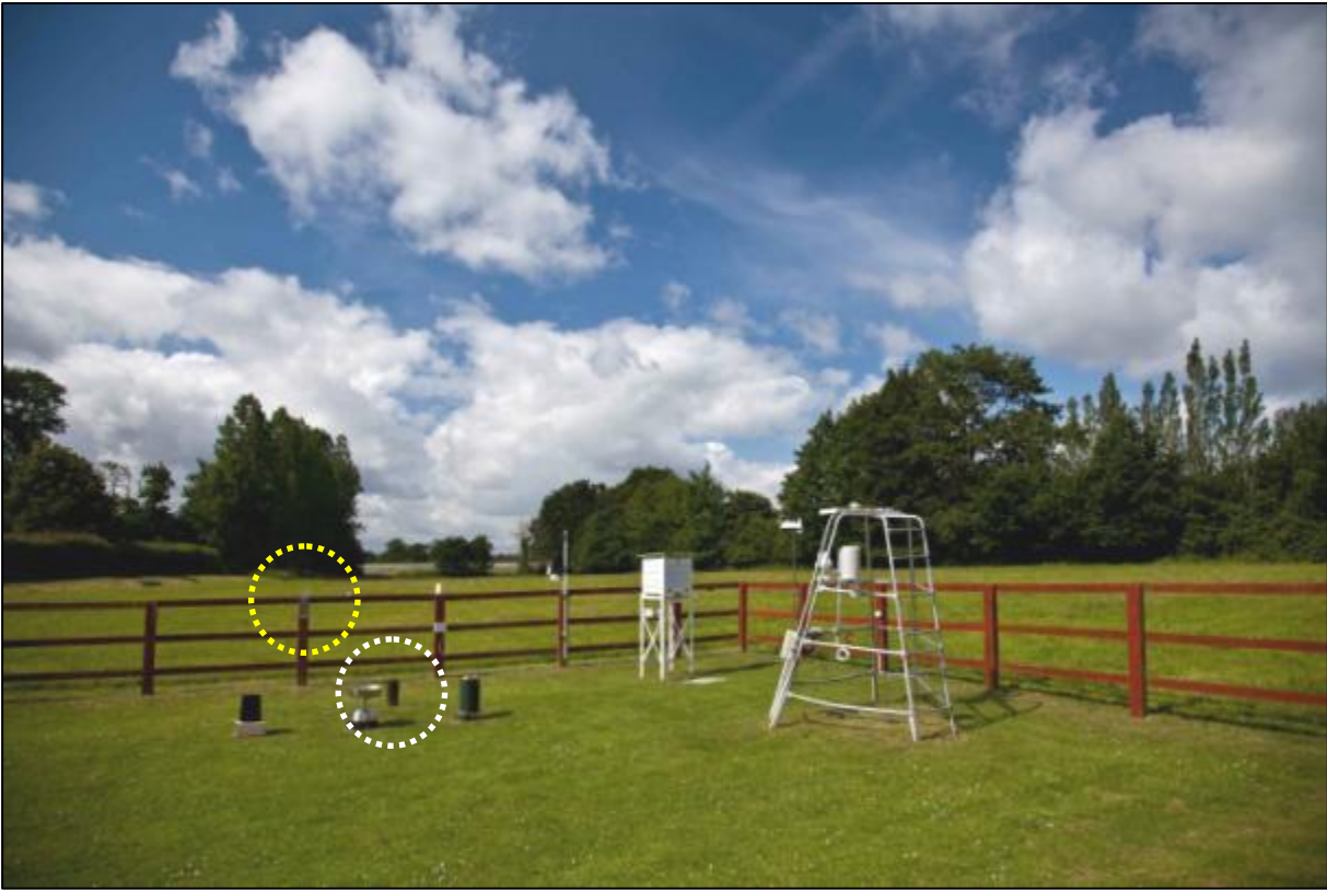
Figure 2 – the trials site in central southern England, looking south-west. The CoCoRaHS raingauge (yellow circle) is located on a fence post at 125 cm above ground level, and 3 metres south of the standard ‘five-inch’ copper raingauge (white circle) used for benchmarking purposes. This photograph was taken on 23 June 2012, shortly after the start of the evaluation period.
